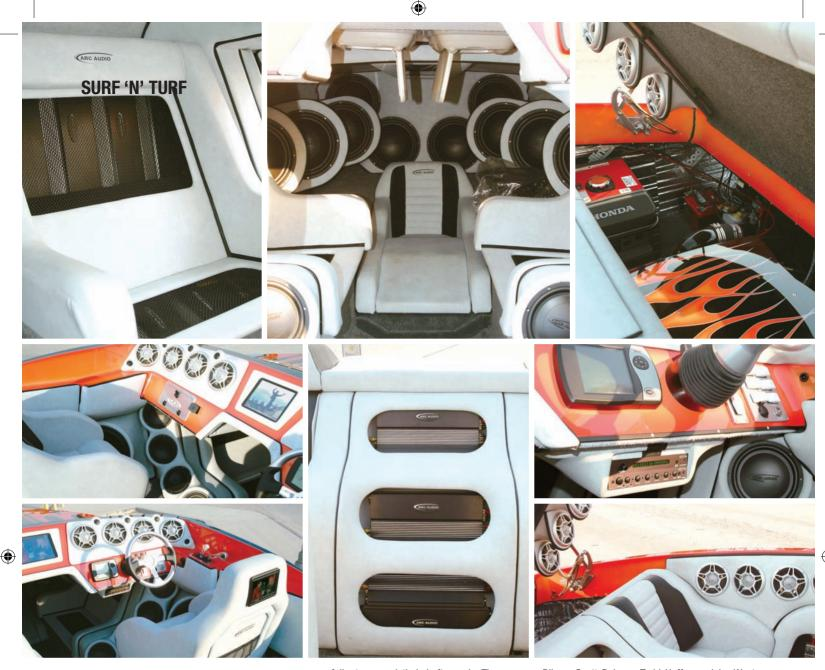
compatible computer with 10.1-inch touch-panel screen, and the rest of the 'dash' features four pairs of Arc's Kar 265 6.5-inch component sets, while down lower, where kick panels would go, are eight Arc 8-inch Dual VC woofers. Two more 15-inch subs pound out the bass when the boat is cruising on the open water.
